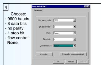
PC is now in terminal mode, connect to device by plugging the RS232 link cable. Measure is now displayed and to access configuration, press **"C"** key .
